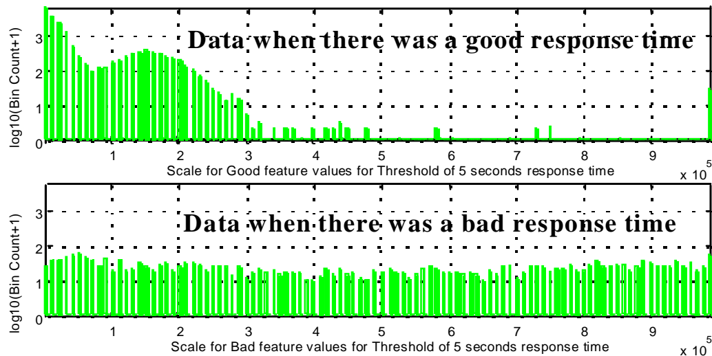
Figure 2. Split Log-Histograms of User CPU Time (msec) for Good and Bad Response Times.
